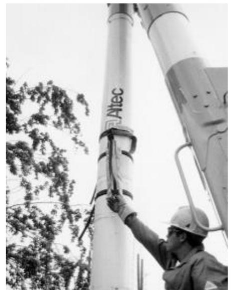
2. Rescuer secures the fall line snaphook to the fall arrest attachment of the lineman's harness and removes his fall arrest lanyard.
