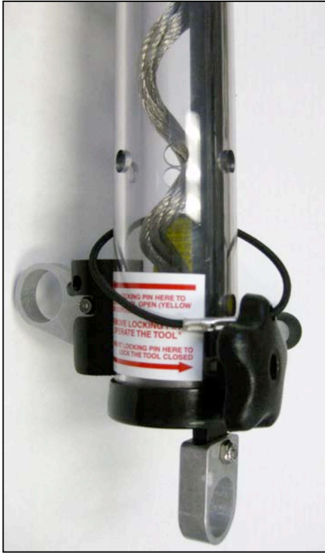
Safety Pin Correctly Installed in the Closed Position.
