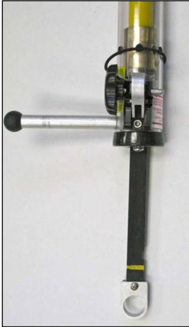
Safety Pin Correctly Installed in the Open Position.
